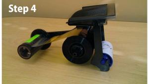
4) Place the assembled cleaning roller back on the ribbon holder using the hooks. The assembly should click into place.
